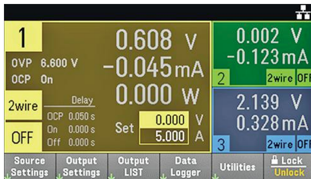
4. The user can view details of a single channel, including the measured power, OVP/OCP condition, and delays.
