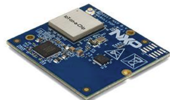
4. NXP's IoT-on-a-Chip SIP combines an i.MX SoC with Wi-Fi and Bluetooth support. The chip is shown here in the upper left of NXP's SOM board.
