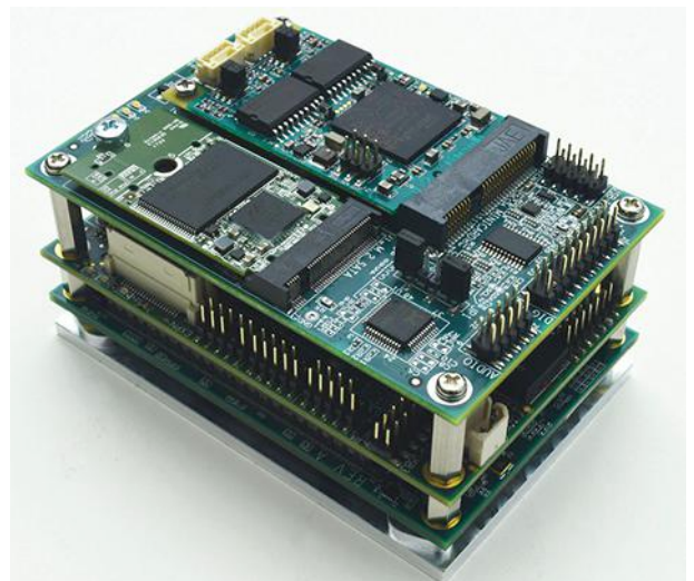
1. Diamond Systems' Zeta COM Express SBC family can work with carrier boards that include Mini-PCIe and M.2.
