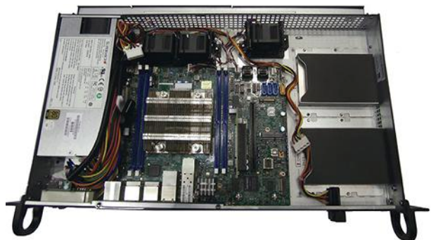
2. Supermicro's 5019D-FN8TP system has a motherboard with an M.2 B Key socket and Mini-PCIe socket that includes mSATA support.
