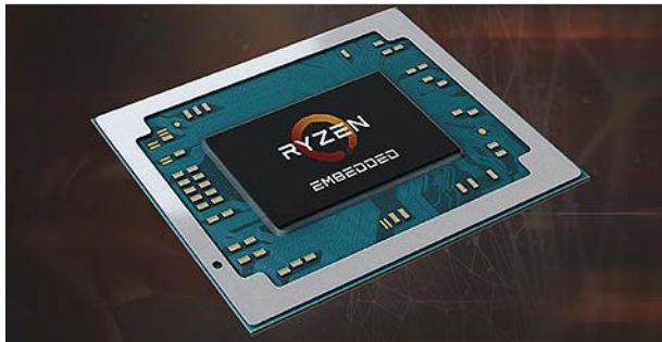
3. Unlike the EPYC Embedded, the Ryzen Embedded incorporates a GPU.
